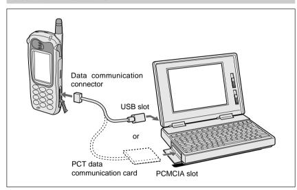
When connected to a personal computer, the display appears in the standby mode.
